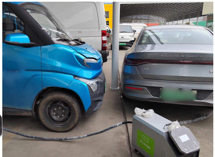
Disassembly design, It is supporting CCS, Chademo and GBT charging standard with only replace the charging gun.
